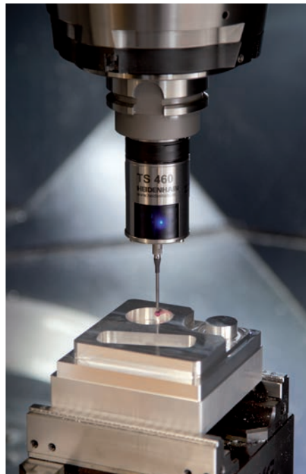
Measuring a circular pocket/hole
